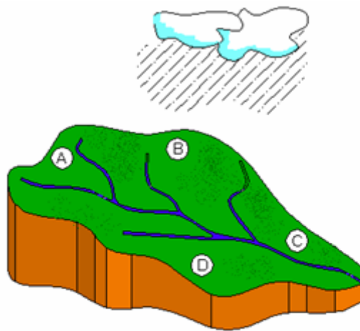
FIGURE 1. A hypothetical catchment showing four rain gauge stations
