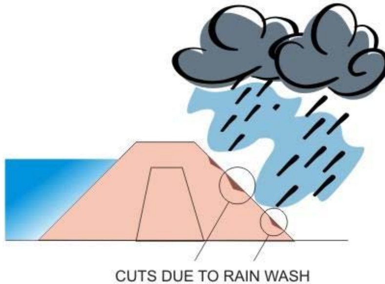
Figure 24. Scour of downstream face by impact of rain and resulting sheet flow
