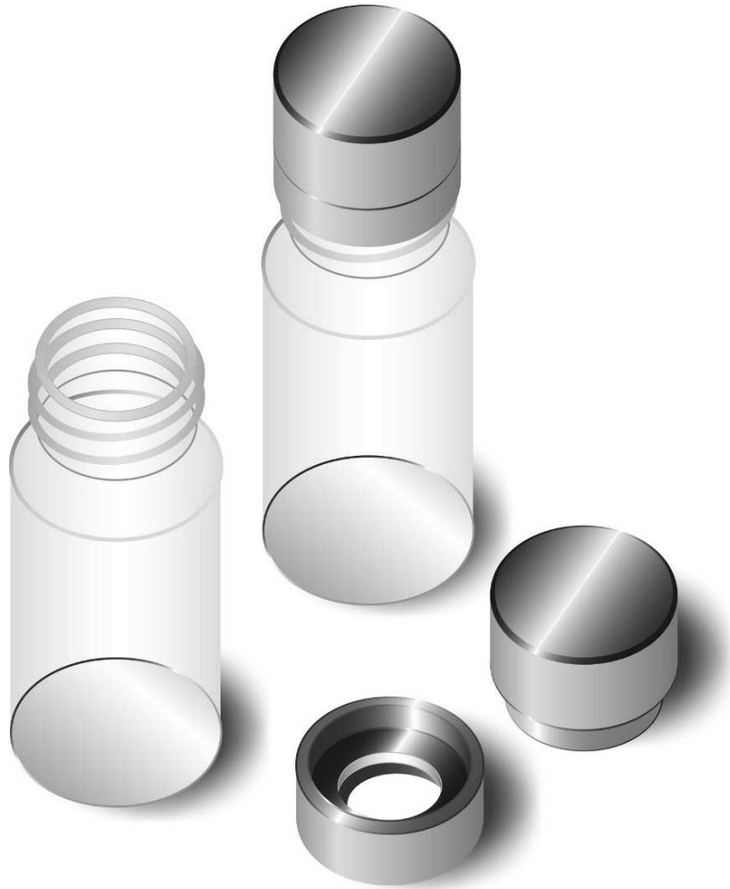
Fig. 9.3 Experimental setup used for measuring the effect of humidity on water permeability. Stainless steel transpiration chambers containing radio-labelled water were mounted upside down on scintillation vials. Inside the vials, various humidities were established using glycerol (2% humidity), glycerol water mixtures (humidity between 2 and 100%) or pure water (100% humidity)
