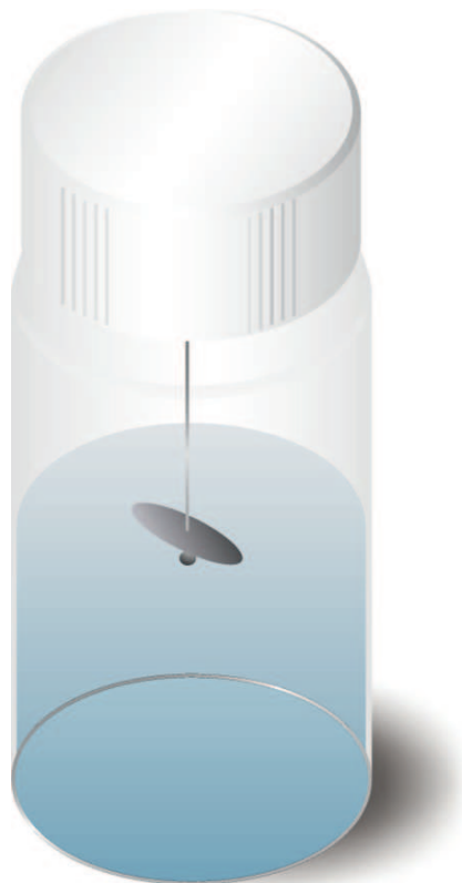
Fig. 9.1 Experimental setup used for measuring sorption or diffusion coefficients. An aluminium disk covered with reconstituted wax was affixed with a needle to the screw cap of a glass vial. The aluminium disk was immersed in an aqueous solution for either loading the wax with a radio-labelled compound (determination of K_{ww} ) or for desorption of a radio-labelled compound from wax (determination of D )
