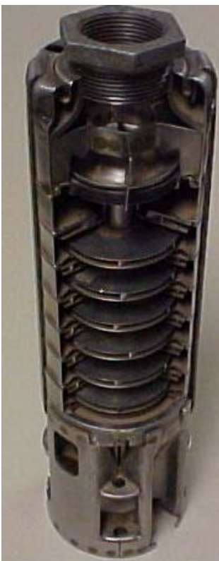
Cut away of a small submersible pump.
