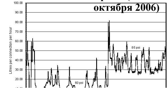
Figure 10: Flow nightline at 5-seconds interval for ductile iron sub-DMA in Orleans on 18 October 2006
