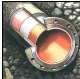
Figure 11 – 13: Pipe before rehabilitation / pipe with impregnated textile tube before heating / rehabilitated
