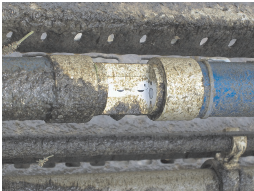
Figure 5. Deposition of sediments can hamper measurement. Cleaning, e.g. using an automated cleaning system is required for proper operations in water with a high fouling potential
