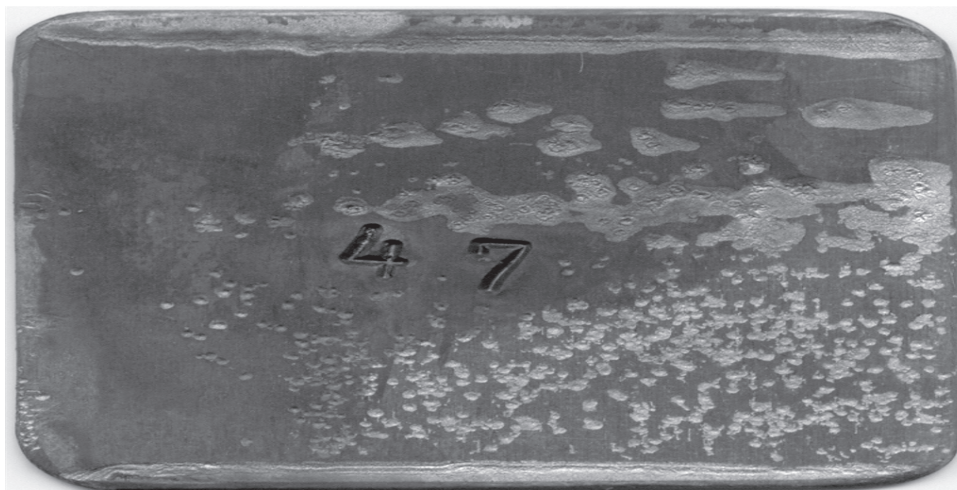
Figure 6. Corrosion coupon after finishing the test – an example of dotted and area corrosion
