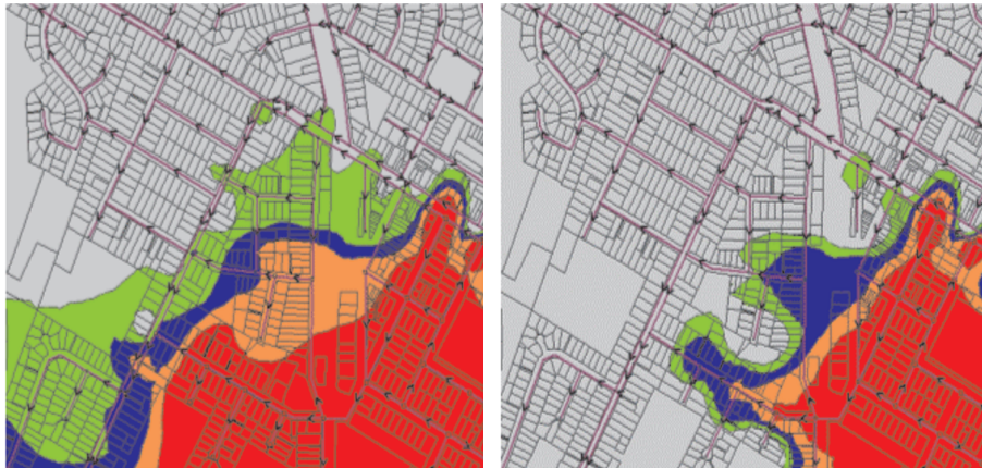
Figure 3. Spreading over time of a pollutant in a water supply system, MIKE NET Software
