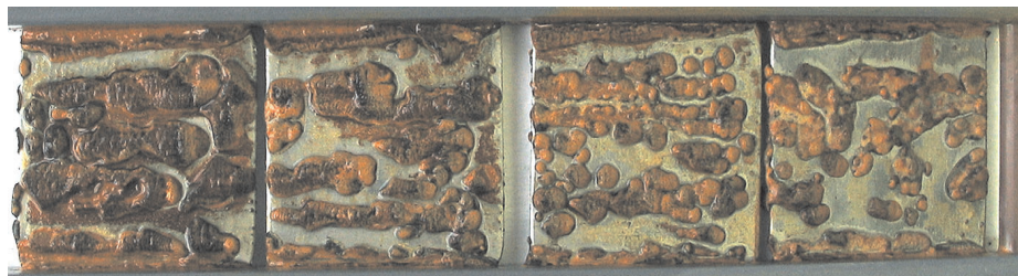
Figure 4. Filtered water – coupons after removal from water – March 8, 2005 (exposure 70 days)
