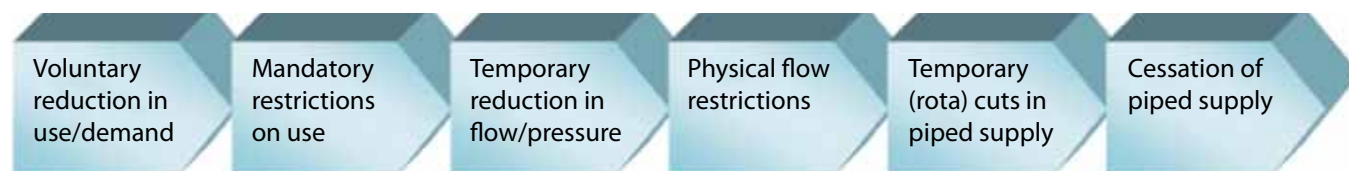
Fig. 11. Intervention options in extreme events (floods)
