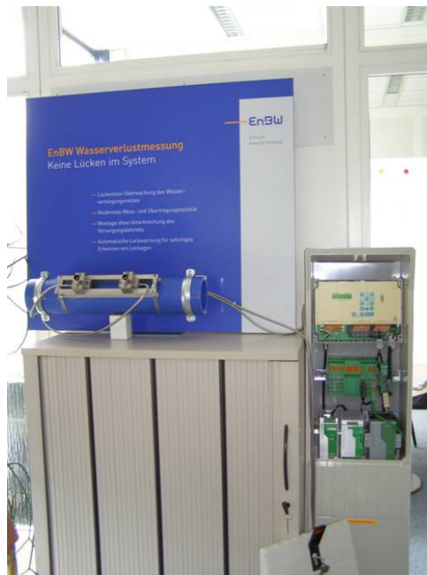
Figure 7: water loss / EnBW-system 'Leak Control'
